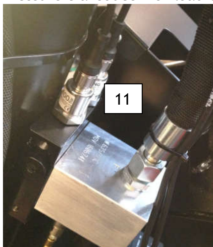
11. Pressure transducer for load control
